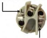
The N terminal is connected with the blue line
