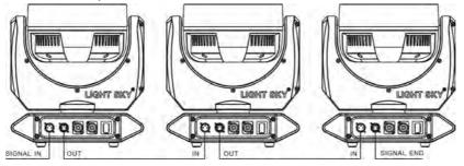
The communicate cable is 2-pin shielded cable  $75\Omega$
